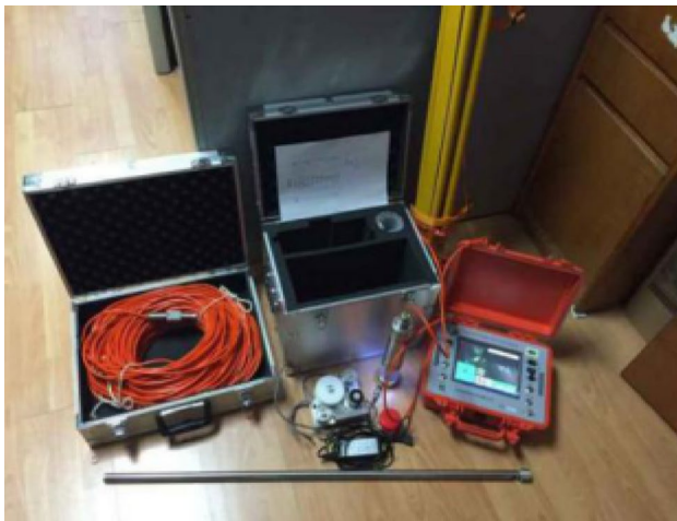
Fig. 14 The digital borehole camera
