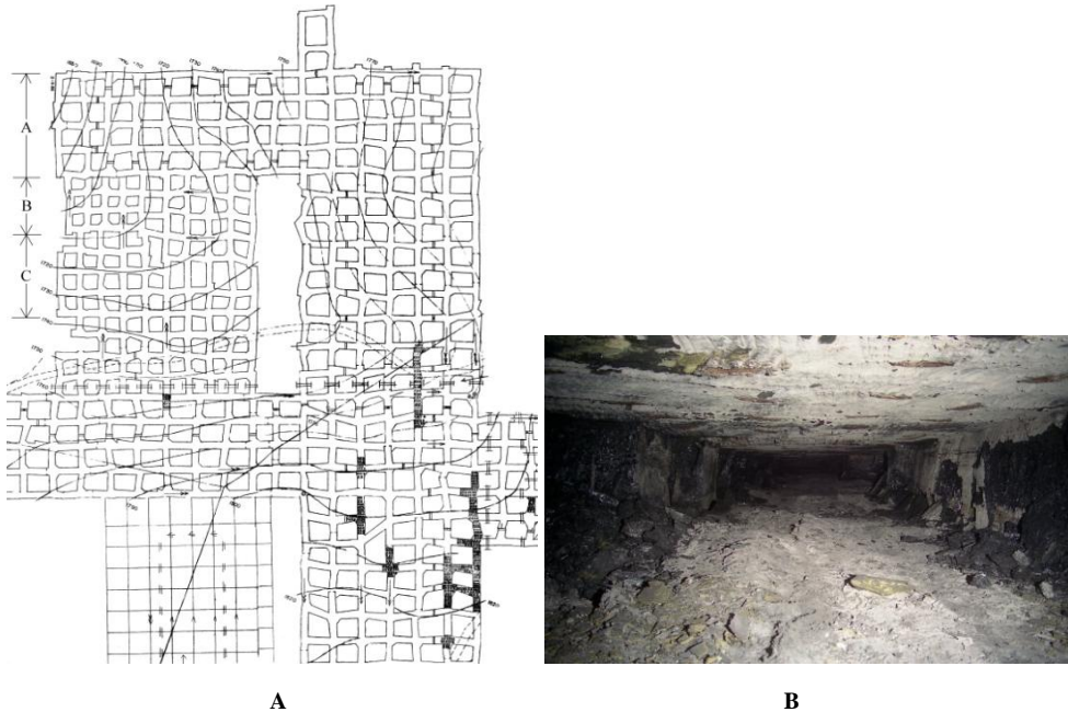
Fig. 5.2.7 A, trial section of pillar design and B, floor heave in the 50 x 50 ft (15 x 15 m) pillar area (Peng, 2007; Peng and Dutta, 1992)
