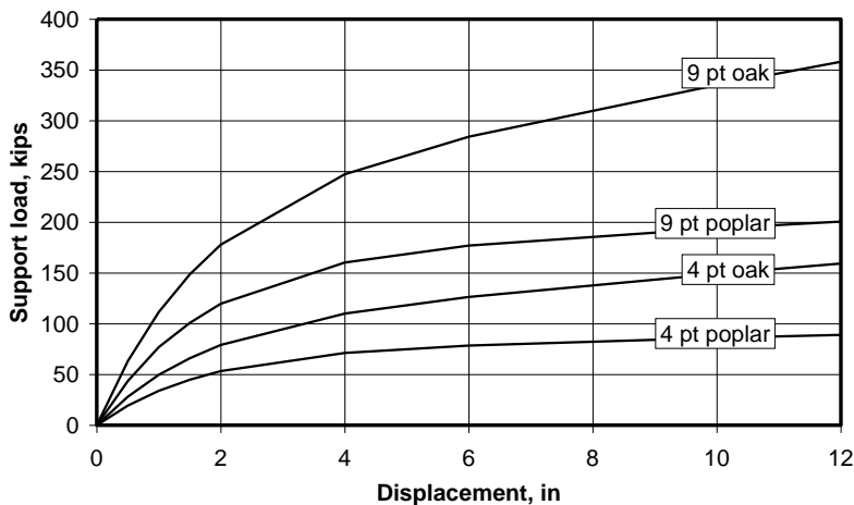
Fig. 7.13.1 Load-displacement curves for conventional wood cribs (Mucho et al., 1999)
