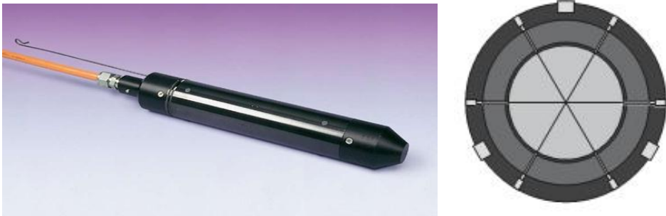
Fig. 11.3.20 Biaxial stress meter (Courtesy Geokon Inc.)
