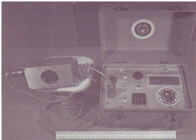
Fig. 11.4.2 Ultrasonic convergence instrument (McVey, 1984)
