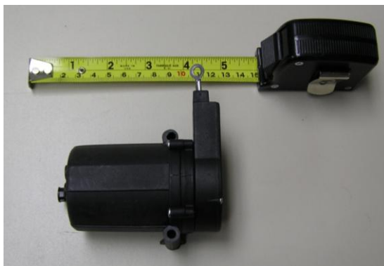
Fig. 11.4.6 Ratiometric potentiometer (Barczak et al., 2008)
