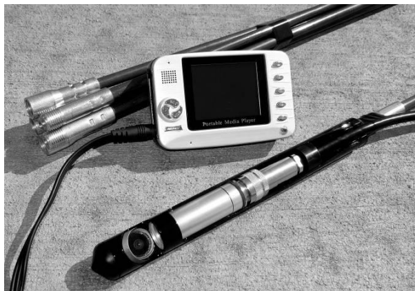
Fig. 11.7.2 FLETCHER borescope (Anderson and Prosser, 2007)
